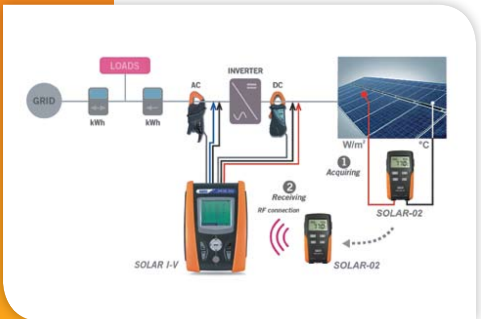
Figure 4. Simultaneous holistic testing of all system components
