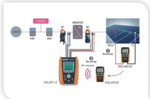
Holistic simultaneous check of PV system components
